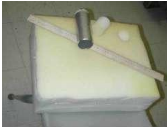
Figure 3 - Piece of foam to create lungs in model. The metallic cylinder was used to create holes for pathologies.
