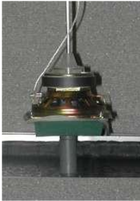
Figure 7 - The electro-dynamic driver in its holder on the model. The green foam is the sound deadening material and the grey plastic cylinder is the striker.
