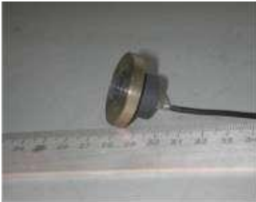
Figure 11 Left: Conical unit with plastic membrane and microphone. Right: Neonatal stethoscope with microphone attached..
