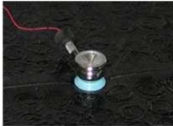
Figure 11 Left: Conical unit with plastic membrane and microphone. Right: Neonatal stethoscope with microphone attached..
